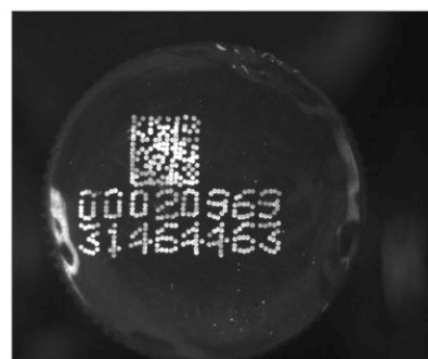
CST-RS7460-UV365 瓶盖隐形码检测
